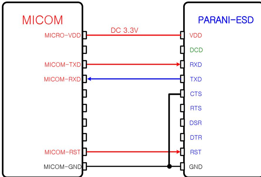
**A.2.1.3. When TTL level of MICOM is 5V**
